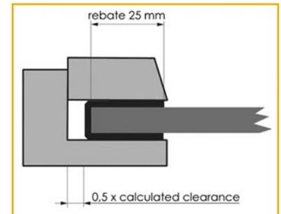
To achieve glazing impermeability to rain water, only sealing agents shall be used which are compatible with acrylic sheet. Construction and sealing material must allow the movement of sheet inside the profiles due to dimensional changes of sheet. Profiled EPDM joints, preferably in white, have proven to be successful in heat loss avoidance. In most cases, profiled joints of non-rigid PVC and PUR foam are incompatible, due to the migration of plasticizers.
