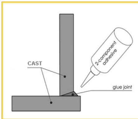
Polymerisation adhesives are also suitable for large and uneven bonding surfaces. Planar bonding is possible.
