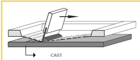
Silk-screen printing is the most commonly used method for printing POLYCASA CAST and allows the creation of a wide range of graphics. Distortion screen printing allows the flat sheet to be formed after printing into a three dimensional article with correct print register. Allowance must be made for “stretching” of the image when designing the graphics.
