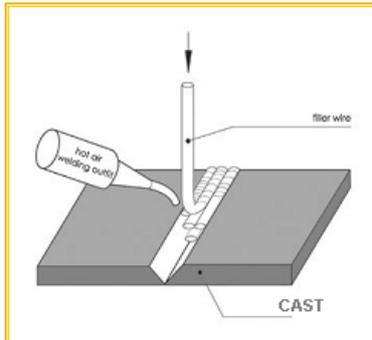
Hot-gas welding is the most frequent welding technique used for POLYCASA CAST sheets.
