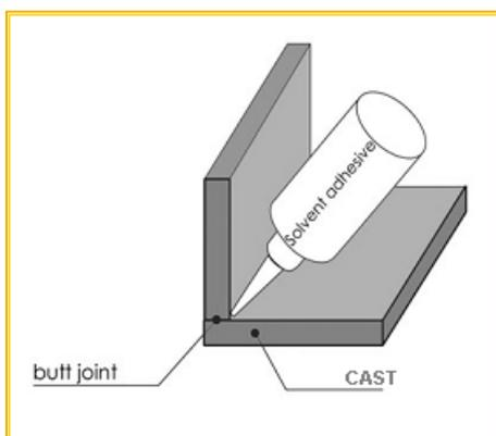
The joint faces must be cleaned prior to bonding. Use warm water containing some washing-up liquid, if necessary; dry with an absorbent, lint free fabric (e.g. glove material). Highly greasy or oily surfaces can be washed with hexane or petroleum ether.
