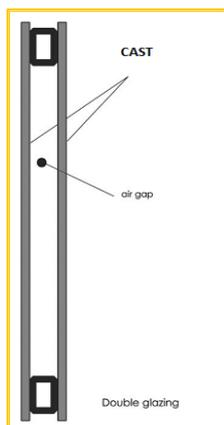
POLYCASA CAST sheets when used for glazing represent considerable energy cost savings as they prevent excessive heat loss in winter and heat intrusion in summer. The heat loss factor of POLYCASA CAST normally referred to as K-value is significantly lower than for glass of the same thickness. The K-value is the parameter which identifies the heat loss of a building with glazed walls.
