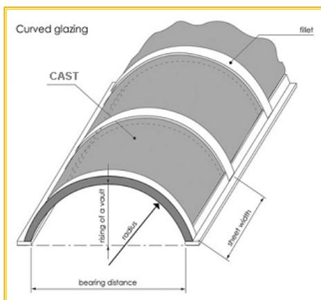
POLYCASA CAST is suitable for cold bending technique. This method facilitates the application of thinner material gauges compared to plane roofing, as an increased self-rigidity of the sheet is achieved due to the change in geometry.
