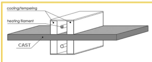
Extended heating is carried out by filaments or heating rods.
