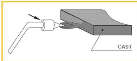
Polish-milling with diamond-tipped tools is another process option. The surface quality is such that no further treatment is required. Polish-milling - in one single work cycle without rough-grinding - will produce excellent finish. No internal stress occurrence; tempering which is essential to other procedures, becomes redundant.
