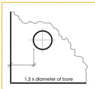
The drilled holes must be adequately dimensioned when fixing to specific points, in order to also allow for a sheet length clearance of 0.07 mm/m °C.
